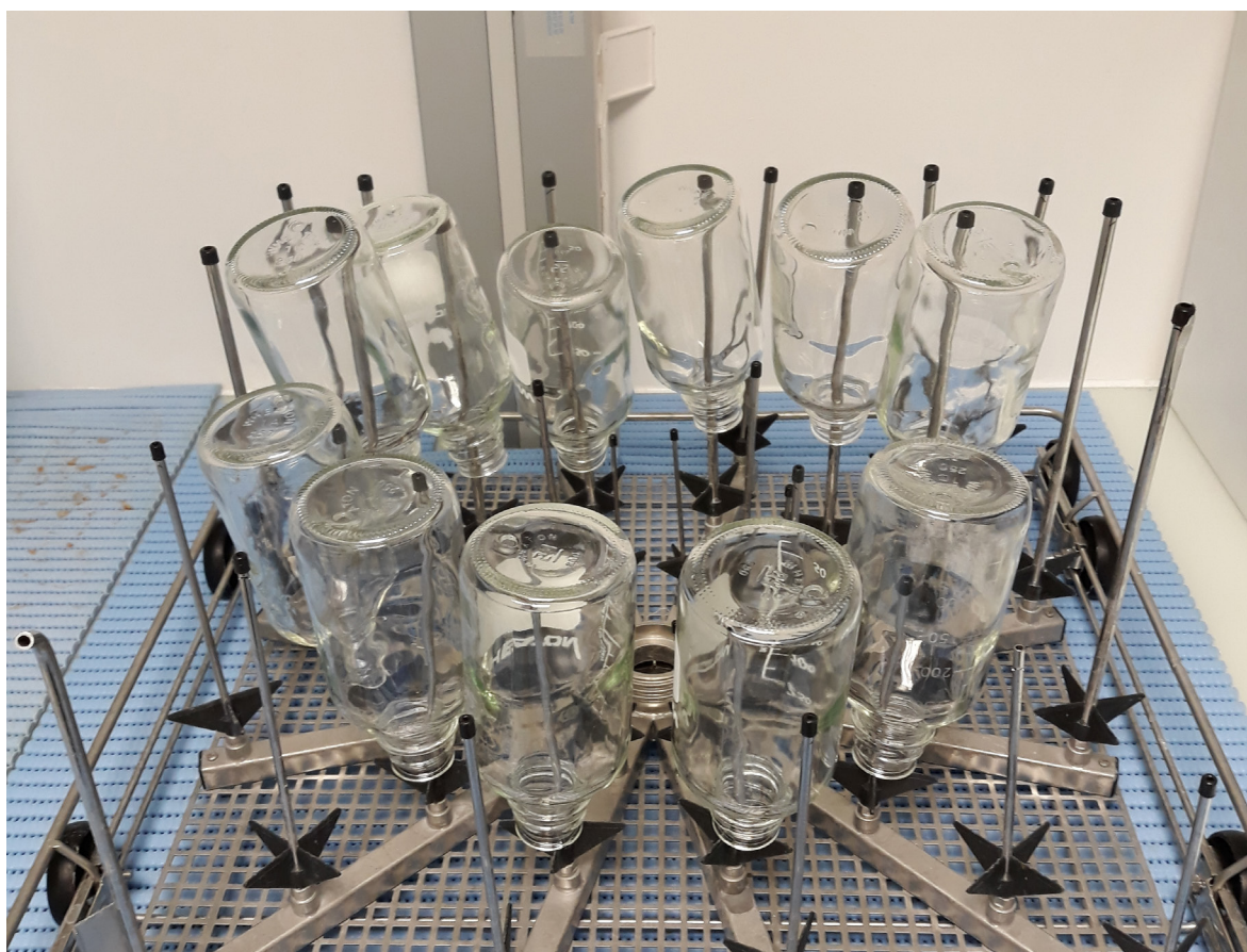
Fig. 5. Method of drying glass bottles upside down on raised steel rods
