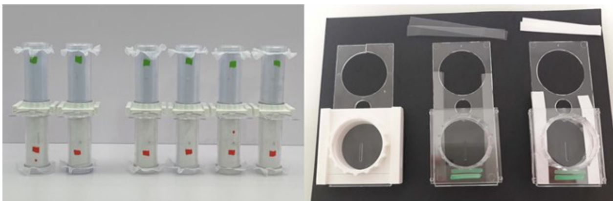
Fig. 5. Examples of modifications that may improve WHO test kits for use with sand flies: using fine mesh screen and the 3D-printed slide unit (left) and inserting thin strips of plastic or paper at the sides of the slide to prevent the escape of sand flies (right)
