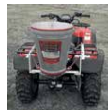
Figure 15. Example of vehicle-mounted rotary spreader
